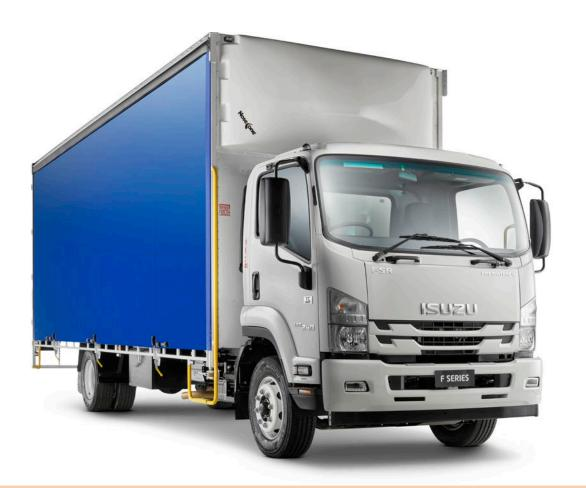
12 pallet (nominal) curtainside body / Easy glide curtains with quick release "Lightning" latches / Lightweight side gates / 3mm chequerplate floor and headboard with load restraints / Safety yellow coloured body steps and grab handles / Underbody mounted storage box / LED lighting for body interior and access steps / Body mounted air deflector / Body interior camera / Isuzu low light capable reversing camera / Daytime running lamps
